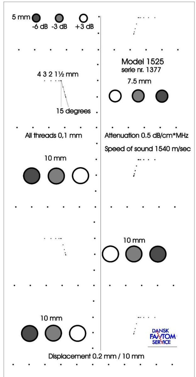
Model 1525 Extra large wire and low contrast phantom for transducers with high penetration
